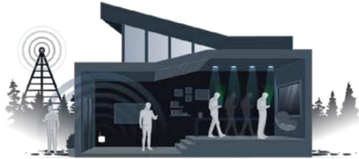
LiFi, like Wi-Fi, enables electronic devices like laptops, tablets, and smartphones to connect wirelessly to the internet. Wi-Fi achieves this using radio frequencies, but LiFi achieves this using the light spectrum which can enable unprecedented data and bandwidth.
